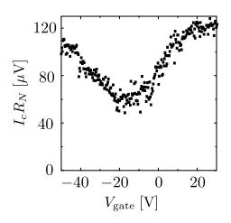
FIG. 15 Product of the critical current  $I_c$  and the normal state resistance  $R_N$  versus gate voltage  $V_{\text{gate}}$ , measured at T = 30 mK in the Josephson junction of Fig. 2. The carrier density in the graphene layer is linearly proportional to  $V_{\text{gate}}$ , while the Fermi energy  $E_F \propto \sqrt{V}_{\text{gate}}$ . The resistance  $R_N$  is measured in the presence of a small magnetic field to drive the electrodes in the normal state. (Heersche et al., 2007)
